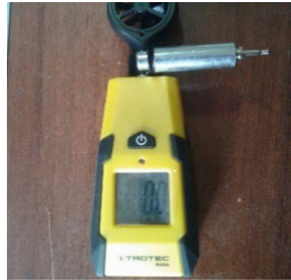
Fig. 2. To measure the speed of the drying agent TROTEC equipment
